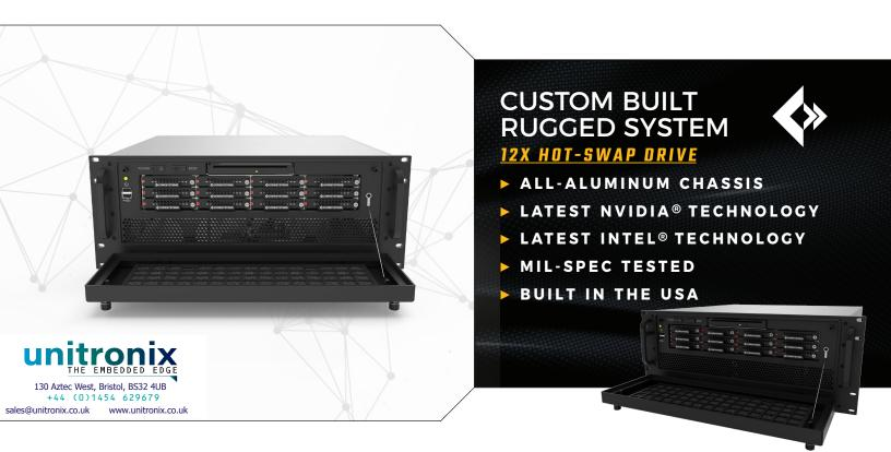
Built with ultra-sturdy all-aluminum chassis, this rugged computer features twelve shock-mounted hot-swap drives and supports the latest Intel® Quad and Hexa-Core CPUs while providing six full-height PCIe slots on the rear of the chassis. The rugged M418 includes the latest single-stack NVIDIA® Tesla® GPU Card which provides our customers with high-performance data analytics and scientific computing abilities.
