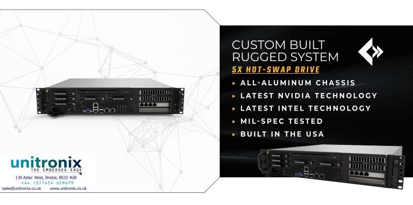
Built with ultra-sturdy all-aluminum chassis, this rugged computer features five shock mounted hot-swap drives and supports the latest Intel Quad and Hexa-Core CPUs while providing a 4-slot front riser card. The rugged M217S-FIO includes the latest single-stack NVIDIA® Tesla® GPU Card which provides our customers with high-performance data analytics and scientific computing abilities.
